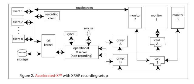
compression is much more effective, and presents a rather simple API for the recording client that will control the recording and playback process. Additionally, clients, including existing ones, do not have to be aware that recording is taking place; it is completely transparent to the normal operating aplications. Only the "Recording Supervisory Client," the small client interface to the X server with the XRAP Extension, is involved.
