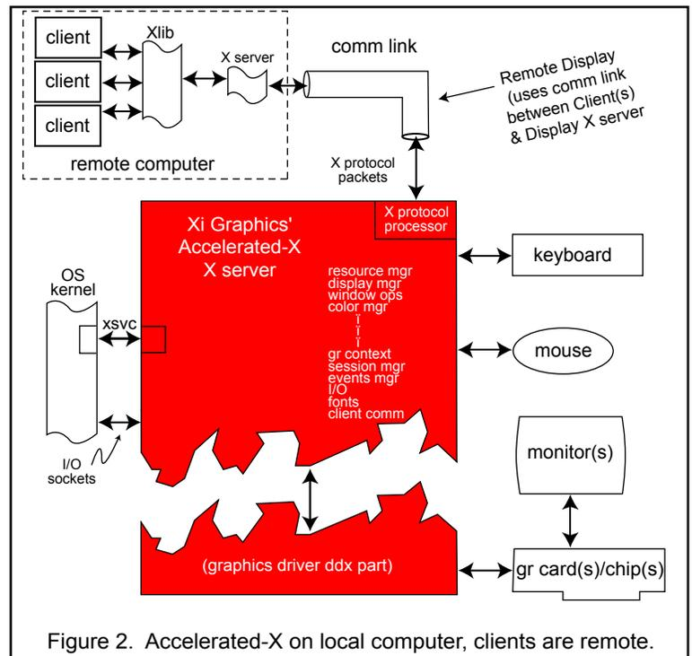
Figure 2. Accelerated-X on local computer, clients are remote.
